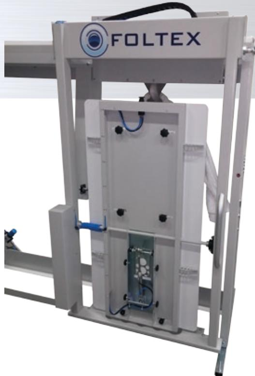
Once the bathrobe is horizontal and the front of the garment is facing down, the operator can manually fold the sleeves so that mechanical blades can create the primary folds and cross fold.
